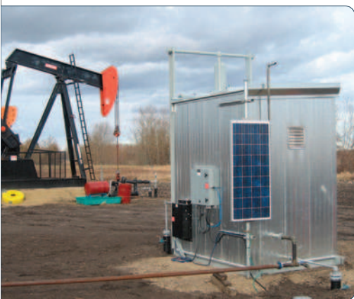
CalScan's Bear solar power control systems can be used either in oil installations (above) or in natural gas environments.
