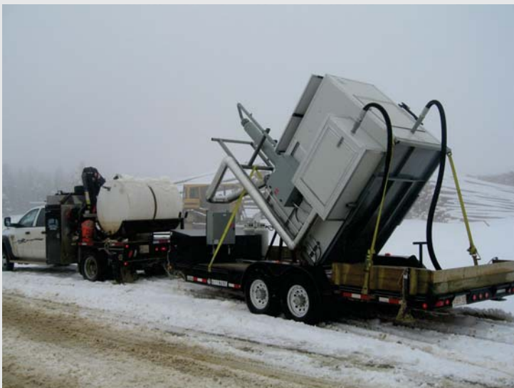
8" Test Separator Configured for Transport
